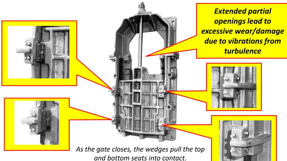
Gate out of turbulent flow when fully open
